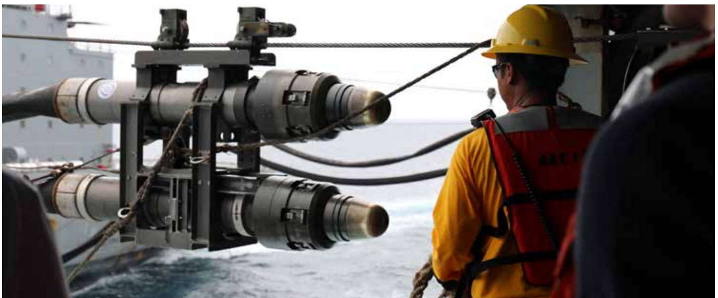
A view of the fuel nozzle from Military Sealift Command's fleet replenishment oiler USNS Kanawha (T-AO 196) as civil service mariners serving on dry cargo and ammunition ship USNS Medgar Evers (T-AKE 13) guide it aboard during an underway replenishment-at-sea. (U.S. Navy photo by Bill Mesta)
